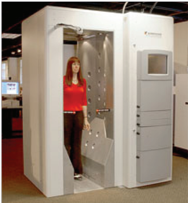
A walk-through portal, developed by Sandia and commercialized by Smiths Detection, is being placed in airports across the country by the Transportation Security Administration to detect trace explosives.
