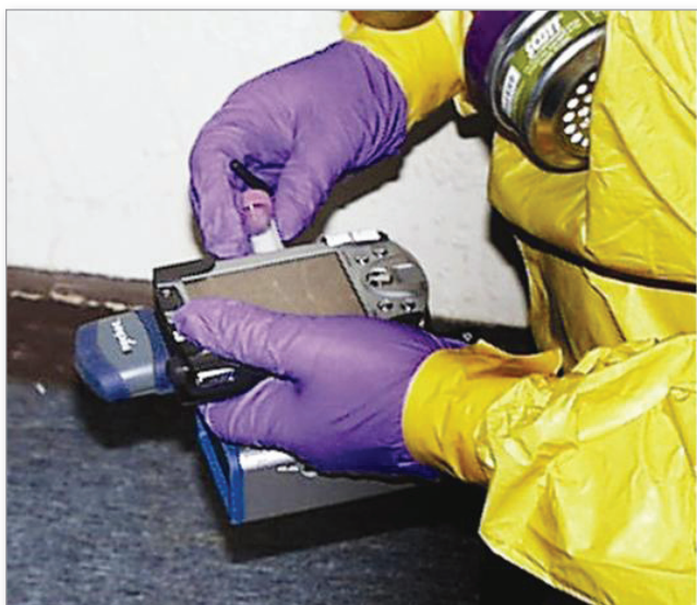
The BROOM system simplifies the process of collecting and processing the many samples needed to restore a facility after a biological attack.
