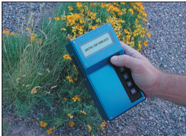
The gas-phase \mu ChemLab system packaged in a battery-powered hand-held unit for portable field use.
