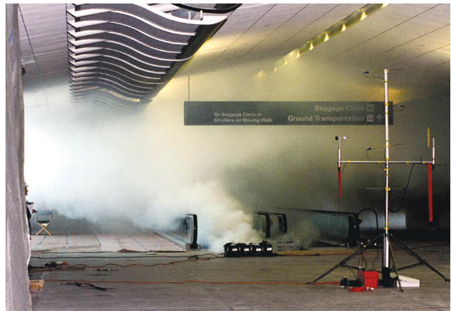
Harmless gases dispatched through SFO's empty international terminal helped the team create evacuation, air handling, and response procedures.
