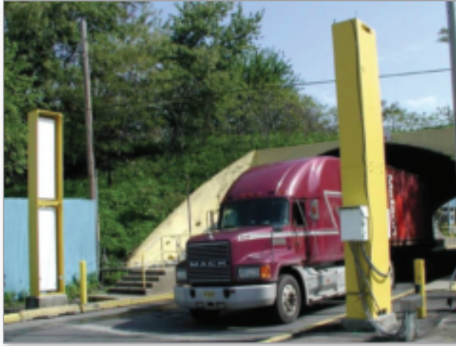
Sandia was instrumental in the Countermeasures Test Bed program to evaluate radiation portals in real traffic at operating shipping facilities.
