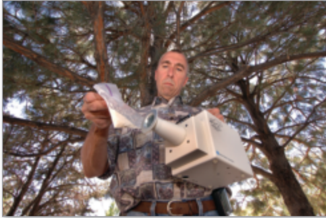
Sandia's Hound device can detect trace amounts of explosives or other chemicals—alerting law and border enforcement personnel of possible malfeasance.
