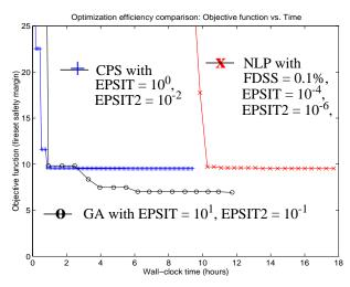
Figure 10. Optimization history for GA runs compared with CPS and NLP starting from (r,x,y)=(1.9, 2.1, 0.0).
