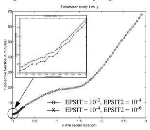
Figure 8. Objective function variation with respect to fire location (y) for r=1.6204 and x=0.78205. Detail shows local nonsmoothness for  $0 \le y \le 0.1$
