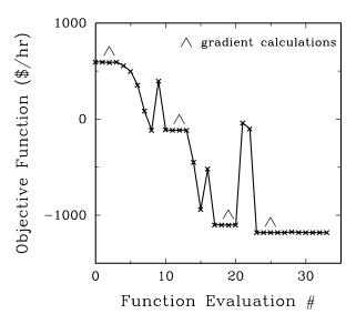
Figure 13. Objective function history for a 3 parameter optimization of a CVD reactor on a coarse mesh. Each conjugate gradient iteration began with a gradient calculation as marked.
