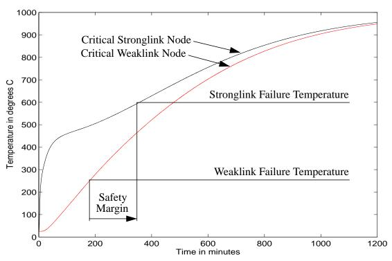
Figure 4. Temperature histories of critical stronglink and weaklink nodes.
