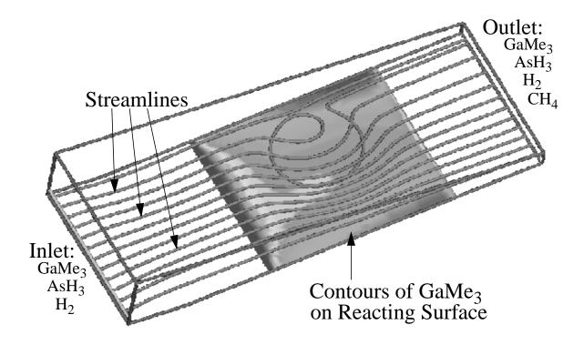
Figure 11. Deposition of Gallium Arsenide in a horizontal CVD reactor with tilted susceptor.
