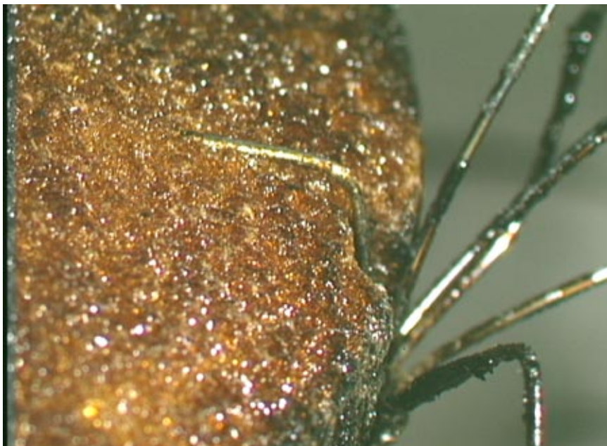
B) Side view of exposed thermocouple
