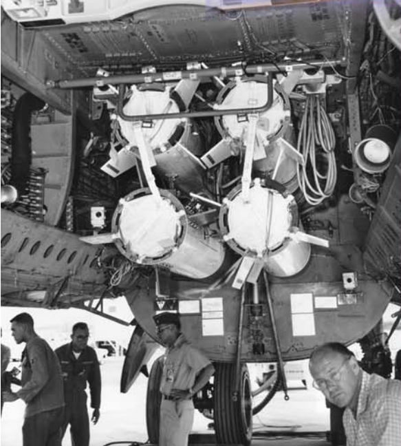
Companion Test Vehicles were used for diagnostic information transmitted to the NC-135s. The number and position of these vehicles varied from test to test.
