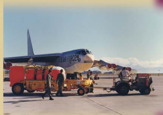
A UTV arrived from the assembly building mounted on its Air Force-designed mobile handling equipment ready to be loaded on a B-52.
