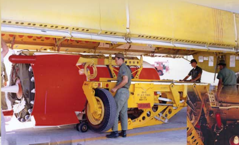
The rear section of a Universal Test Vehicle (UTV) protruded into a free space chamber as part of the pre-B52 loading systems checkout in the assembly building at Barbers Point. Sandia test vehicles (ballistic shapes with arming and fuzing systems) could be tailored to house test devices of various sizes and shapes.
