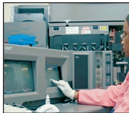
The analyst sets up the flow cytometer for a sorting operation using touch-screen options.
