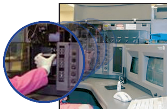
Loading a 96-well microtiter plate for cell sorting with the EPICS® Altra flow cell cytometer.
