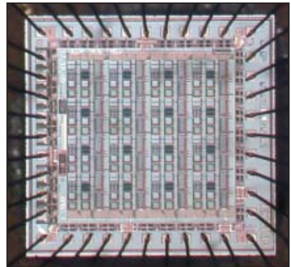
Integrated circuit with photodetector array, built at Oak Ridge National Laboratory
