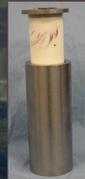
TufFoam™ encapsulant remains intact after testing at 5,000 g's.
