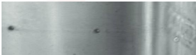
Two picoliter drops are ejected at 10 m/s and 1 KHz using an electrostatic drop ejector fabricated in Sandia's surface micromachining MEMS technology.
