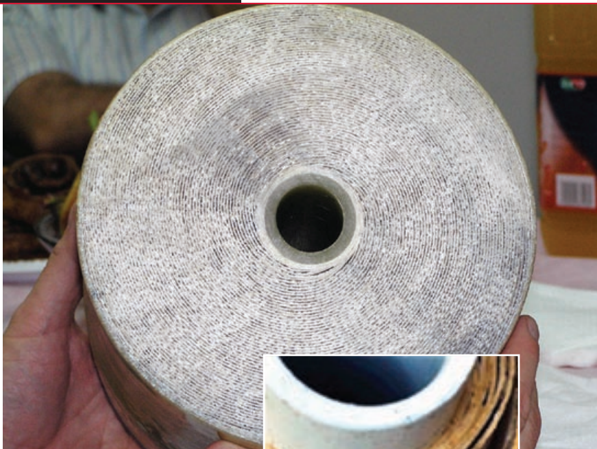
Photos illustrate a typical reverse osmosis filter (top) and fouling problems (bottom).
