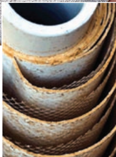
Photos illustrate a typical reverse osmosis filter (top) and fouling problems (bottom).
