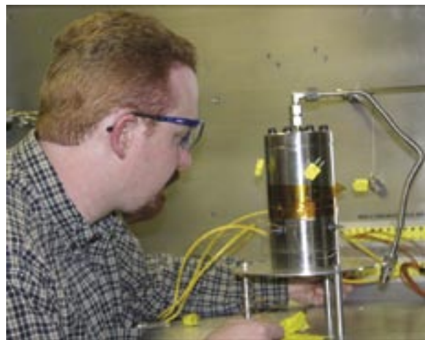
Sandia engineer Mark Zimmerman integrates a hydride bed with temperature monitoring sensors to study recharging and discharging of hydrogen. (Photo by Bud Pelletier)
