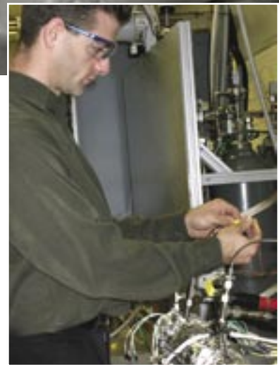
Recharging and release of the hydrogen from metal hydrides require heat, which can reduce overall fuel economy. Sandia engineer Terry Johnson sets up a test apparatus. (Photo by Bud Pelletier)
