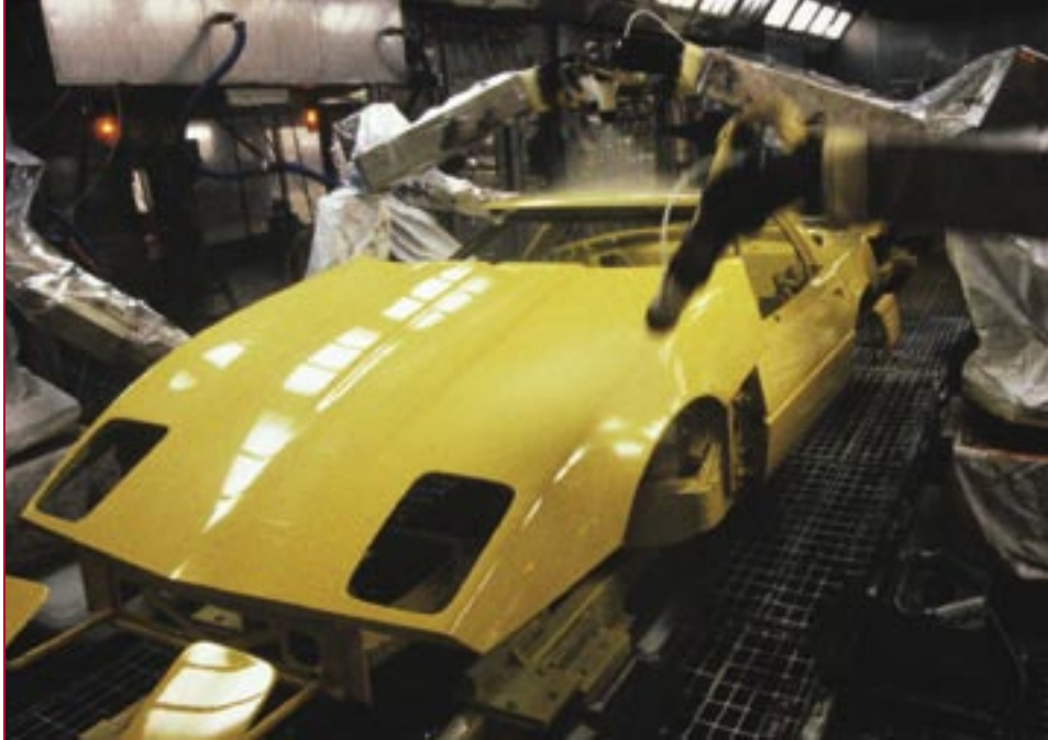
Sandia researchers are working with PPG Industries to improve automotive clearcoat application
