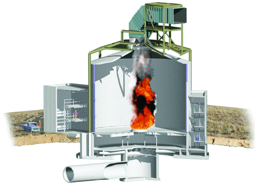
A seven-story FLAME Test Cell is a key part of the new Thermal Test Complex, now under construction at Sandia. The cell includes water-cooled walls, an airflow control system, and high-tech emission filters.
