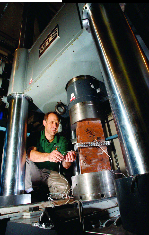
Dave Bronowski (above) and Ron Price (below) study fracture properties of Yucca Mountain's rocks in their Albuquerque laboratory.
