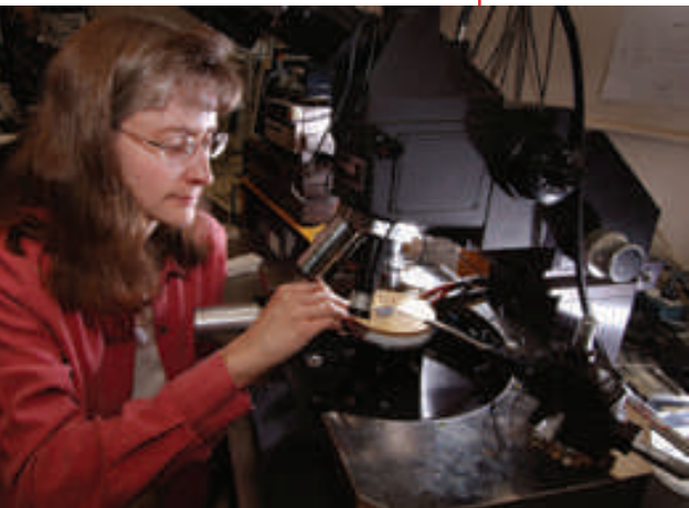
Mary Crawford tests the output of one of Sandia’s newly developed ultraviolet light-emitting diodes.
