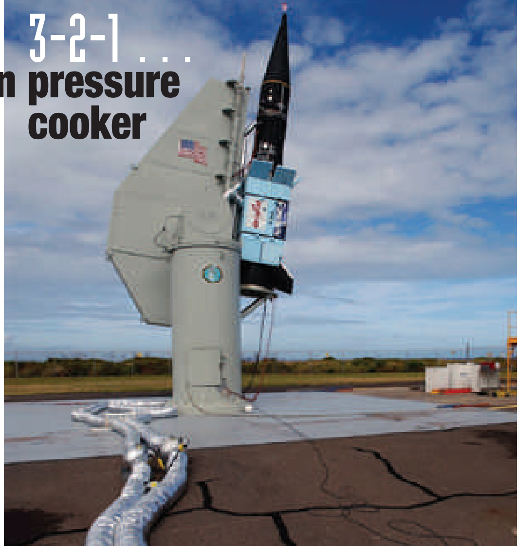
FM-5 target missile on Pad 1's rail launcher ready for liftoff. The flexible conduit supplies cold air to a fall-away cooling chamber, which keeps critical electronics cool until launch.
