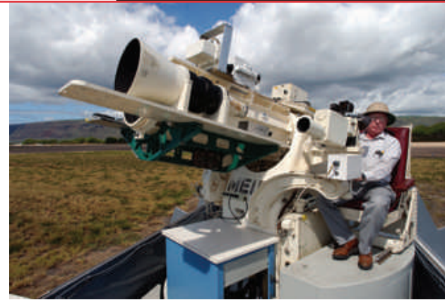
Hovey Corbin in the saddle of an ME-16 tracking telescope one mile south of Pad 1. The ME-16 follows the rocket's trajectory shooting video and pulling film at 100 frames per second.
