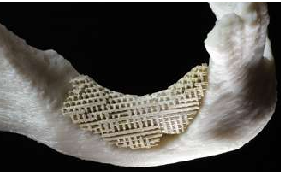
Perfection regained: the perfect fit of the Sandia ceramic scaffolding in the model jaw also recreates the upper line of the original jawbone. The scaffold layerings, which criss-cross each other, expedite passage of new bone and blood vessels. (Photo by Randy Montoya.)
