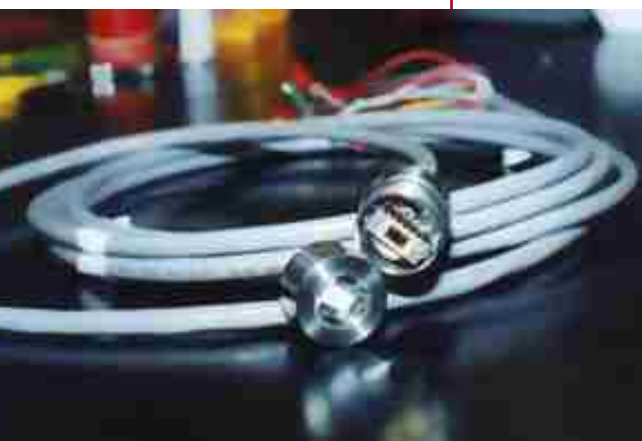
Chemiresistor sensor housing and cable.
