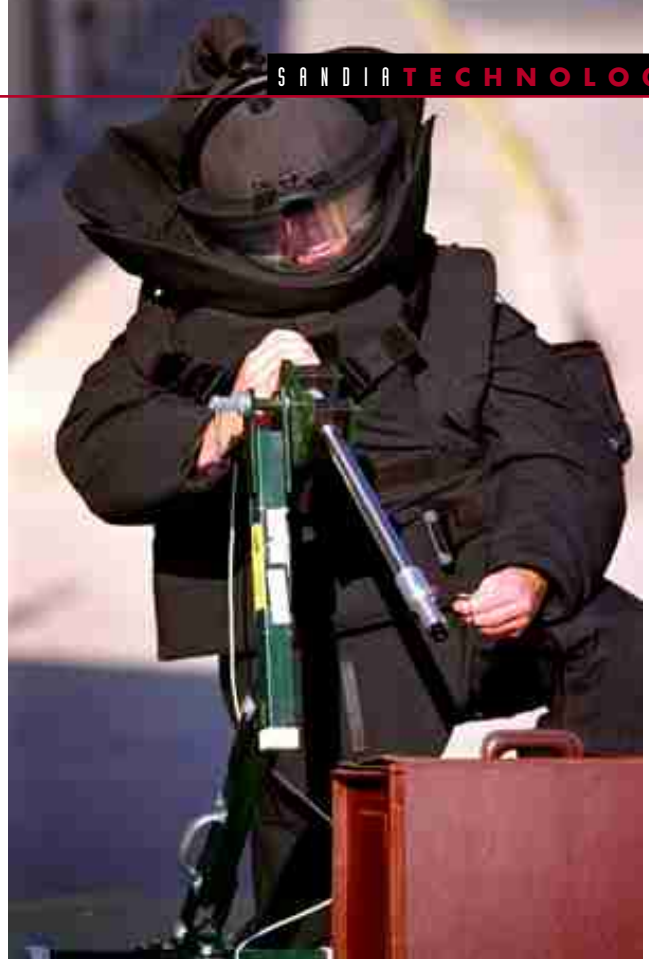
Bomb tech in protective gear uses PAN® disrupter on mock briefcase bomb.
