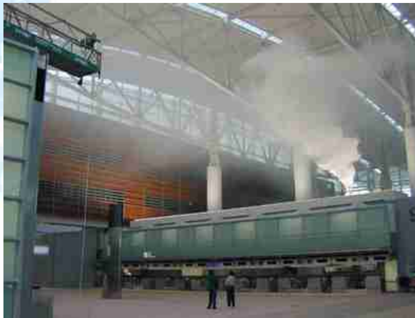
Sandia conducted smoke tests like this to help model airflows in the new SFO International Terminal.
