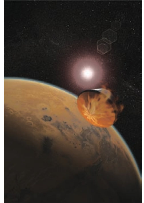
Artist concept of a spacecraft using aerocapture to enter an orbit around Mars. (Image courtesy of NASA)
