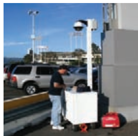
Chemical detection system can detect chemical warfare agents as well as common toxic chemicals.
