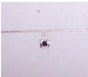
Figure 3: A COTS radio frequency ID tag embedded in 100 \mu\text{m} wide silver antenna lines directly written on a flexible substrate. Mating a tuned antenna to this COTS chip enhanced the range of activation of the chip significantly.
