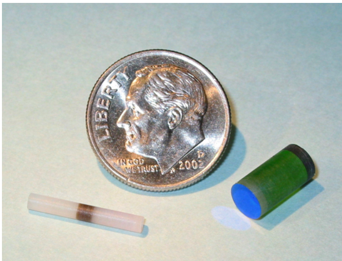
Figure 2: Examples of Sandia-designed microlasers. The microlaser on the left is a Nd:YAG laser designed to produce high-energy ( >200 \mu\text{J}/\text{pulse} ) single-frequency output for spectroscopic applications. The microlaser on the right is a Cr:Nd:GSGG laser which is fabricated from radiation-hard materials and is intended for weapons applications such as optical triggering of sprytrons.
