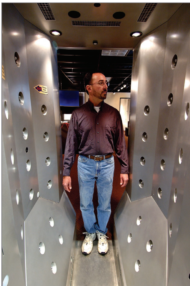
The Sentinel, the commercial version of Sandia's explosives detection personnel portal, puffs air on occupants to dislodge particles for chemical analysis. In TSA's extensive pilot program, the Sentinel screened passengers at several major U.S. airports, including New York's John F. Kennedy International Airport.
