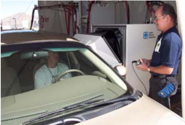
A previous field test of the vehicle portal prototype used two modules (driver's side door and back of vehicle) to test for explosives
