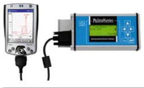
Fig. 6 Photograph of PDA-controlled potentiostat for use with ElectroNeedle™ array.
