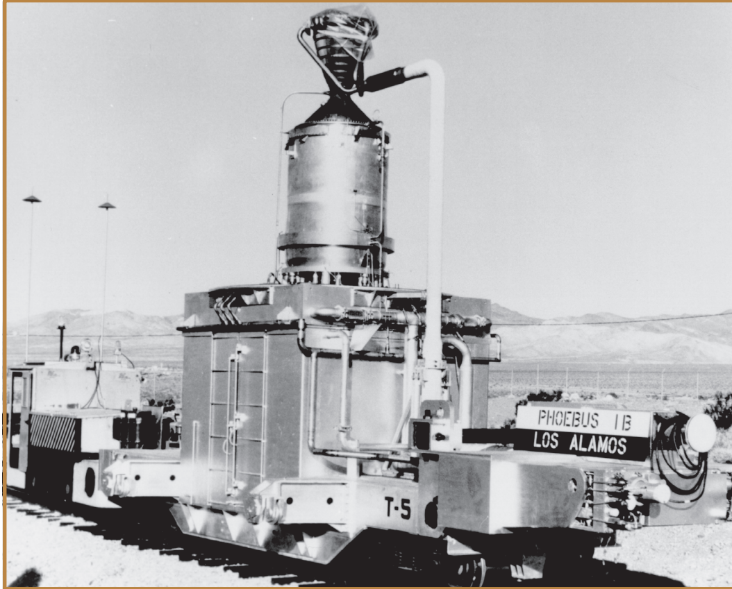
Pictured is the Phoebus 1B reactor mounted on a test cart en route to the Nuclear Rocket Development Station at the Nevada Test Site. The Phoebus 1B was one of 23 nuclear reactor rocket engines tested in the 1960s as part of the space propulsion program.
