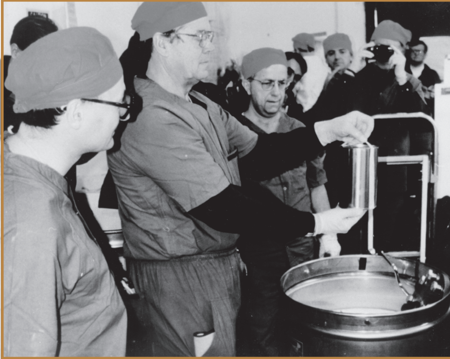
Kazakhstan HEU was packaged into 55-gallon "6M" shipping containers by DOE personnel for shipment to the U.S.
