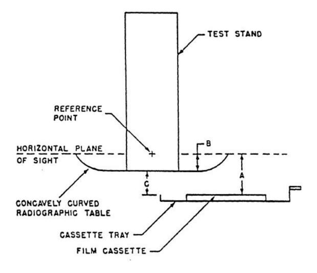
FIGURE 1: HOW TO DETERMINE DISTANCE FROM TOP OF CASSETTE TO BASE OF TEST STAND FOR CONCAVELY CURVED TABLE TOP.  $\label{eq:C} C = B-A = DISTANCE \ FROM \ TOP \ OF \ FILM \ CASSETTE \\ TO \ BASE \ OF \ TEST \ STAND.$
