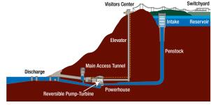
During periods of low power demand, the pump-turbine pumps water up into the mountaintop reservoir. During periods of high demand, water from the mountaintop reservoir flows into the penstock, or large pipe, to the turbines and generator, spinning them to produce electricity in the underground power plant.
