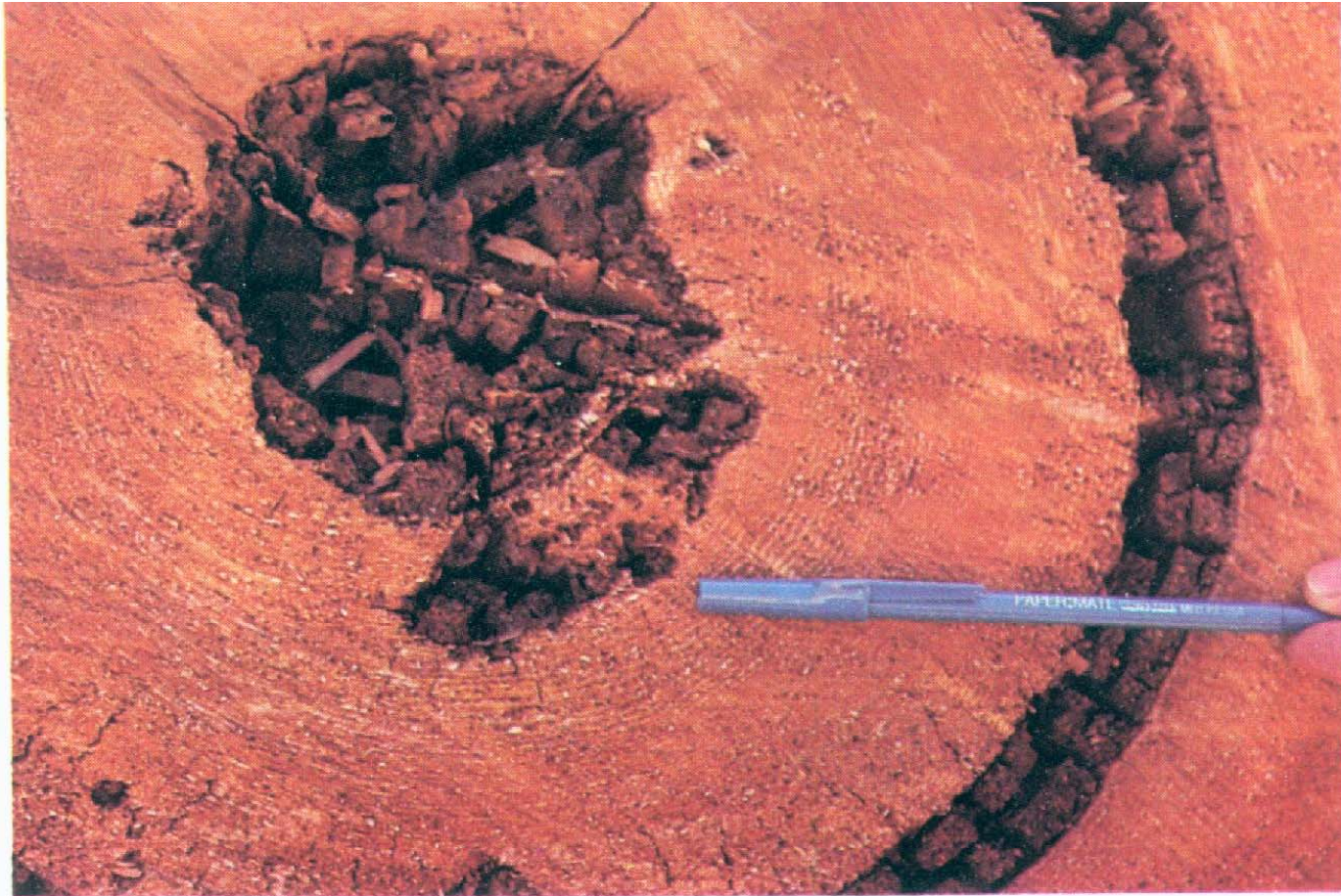
Figure 4. CEDAR BROWN POCKET ROT in western redcedar log decays large pockets.
