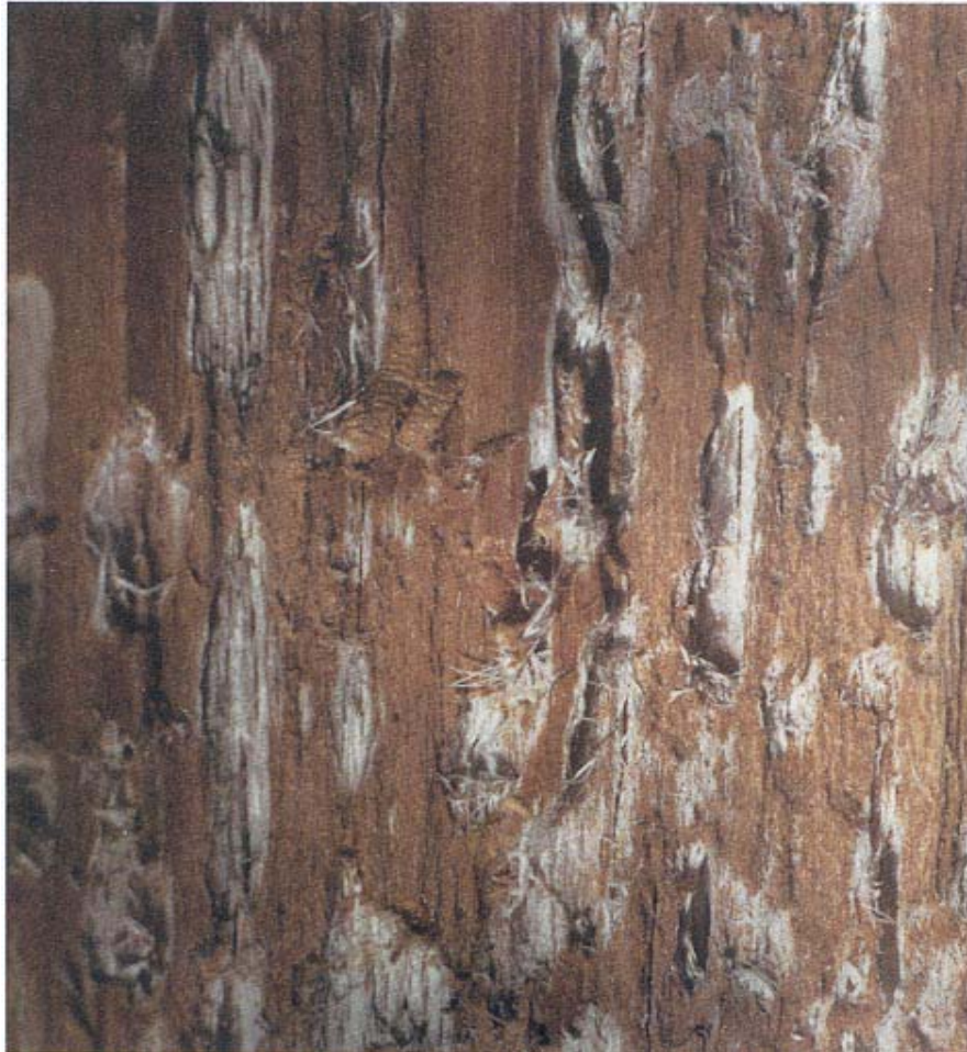
Figure 7-13— White pocket rot of Douglas-fir caused by the red ring rot fungus (Phellinus pini).
