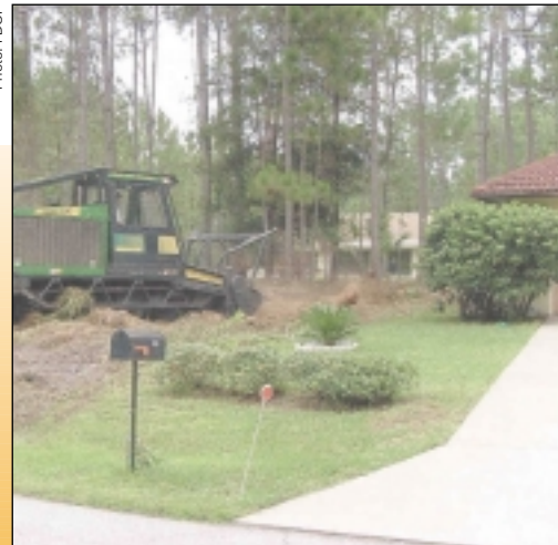
Fuel reduction treatments should be performed on undeveloped lots in subdivisions in high-risk areas. This Gyrotrac® is mowing and chopping heavy fuels in an undeveloped lot of the Palm Coast subdivision in Flagler County, Florida.
