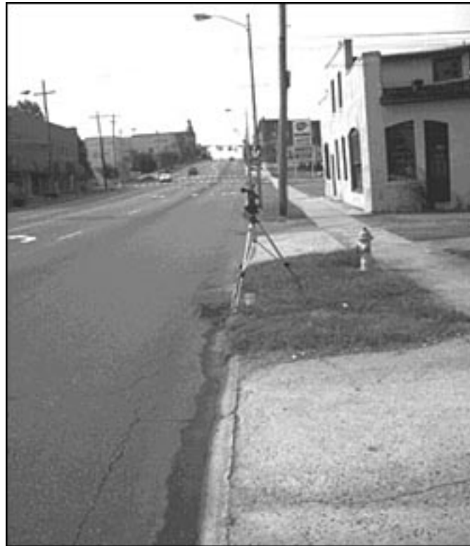
Figure 18. For the intersection study, the camera was positioned upstream of the intersection to allow participants to observe the approach speeds and lane-changing behaviors of motorists.
