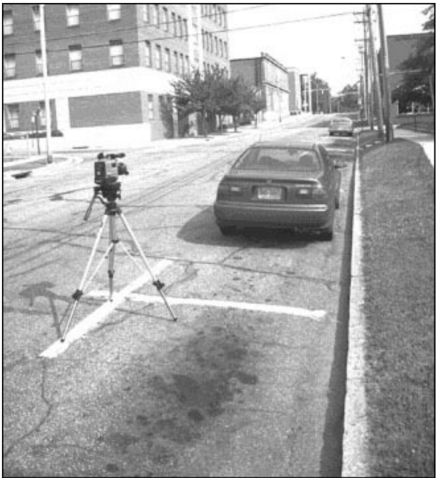
Figure 9. At locations with on-street parking, the camera was positioned at the left edge of the parking lane as close to the travel lane as possible at a height of 1.4 to 1.5 m with the lens aimed parallel to the roadway.
