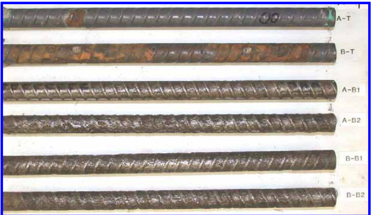
Figure 86. Slab #14 after autopsy
