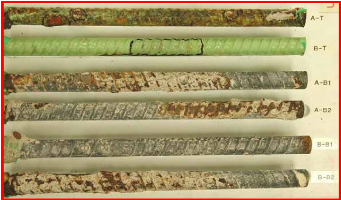
Figure 52. Slab #3 extracted rebar condition
