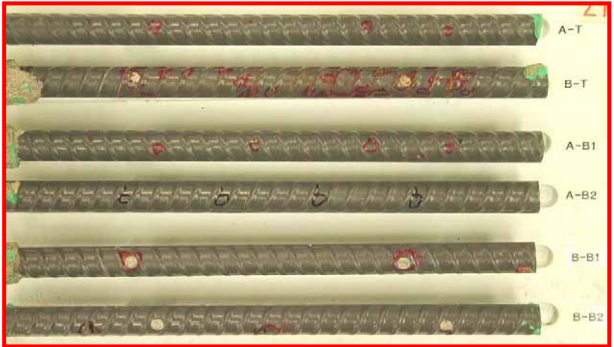
Figure 130. Slab #29 extracted rebar condition
