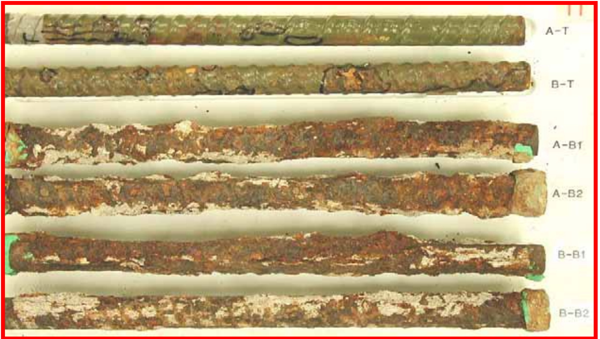
Figure 110. Slab #19 extracted rebar condition
