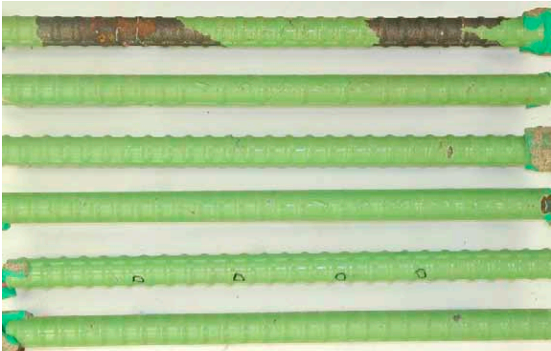
Figure 38. Photograph of autopsied bars extracted from slab #10 (ECRs in both mats)
