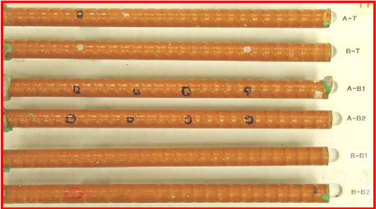
Figure 94. Slab #17 extracted rebars condition
