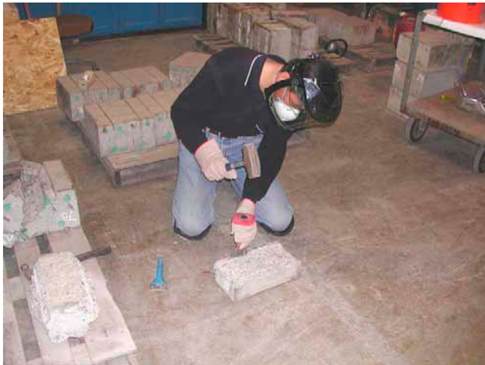
Figure 28. Extraction of embedded reinforcing bars
