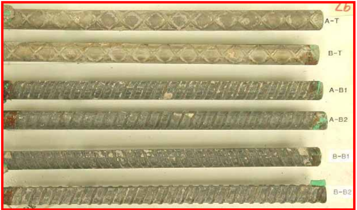
Figure 121. Slab #26 extracted rebars condition
