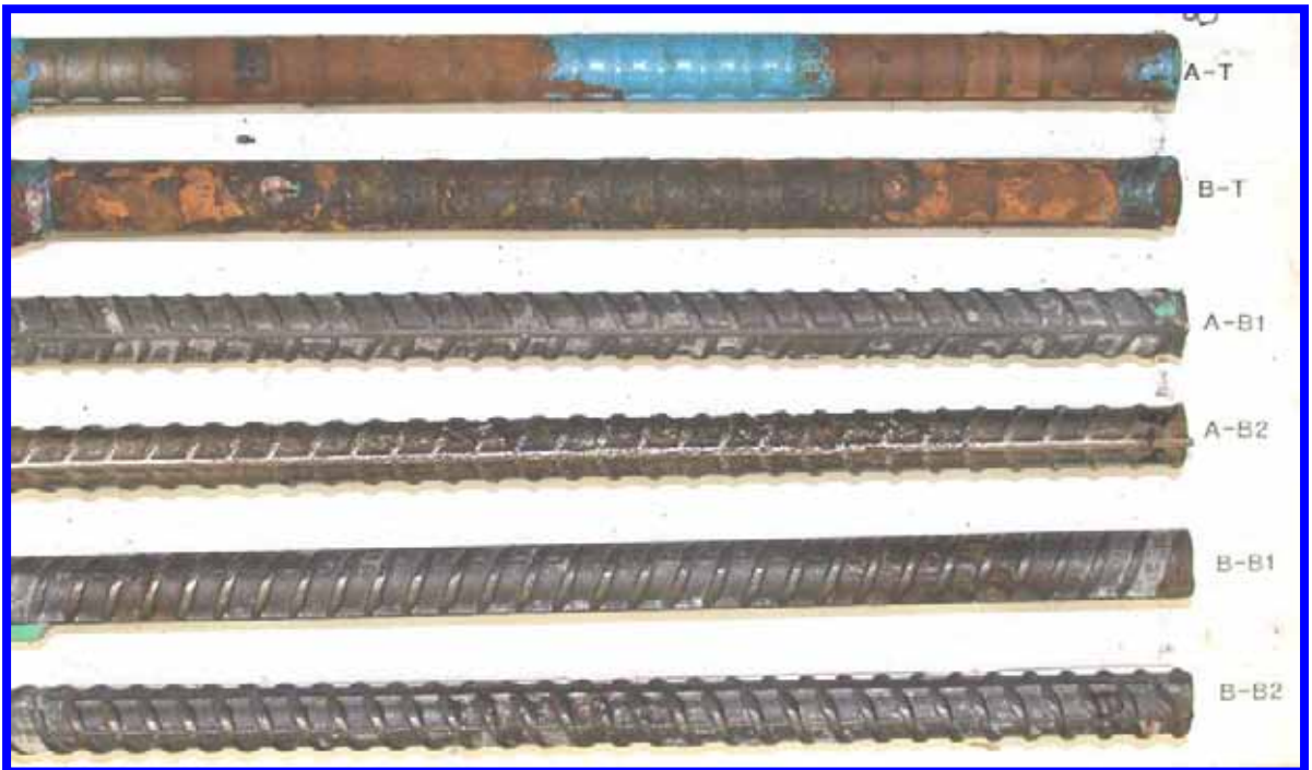
Figure 119. Slab #25 after autopsy
