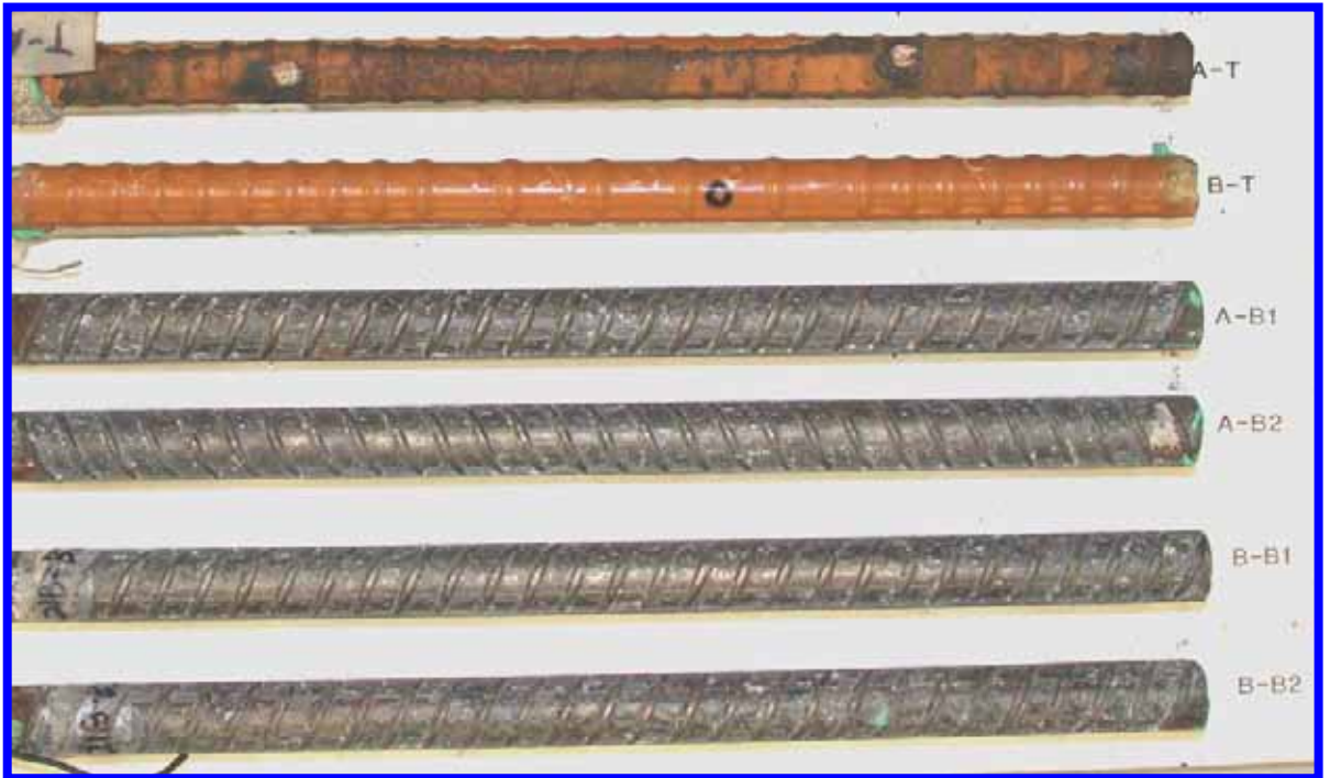
Figure 107. Slab #21 after autopsy
