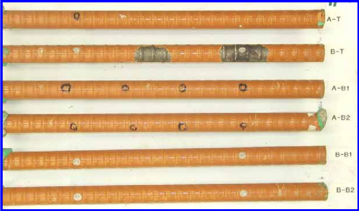
Figure 95. Slab #17 after autopsy
