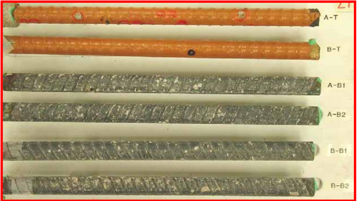
Figure 106. Slab #21 extracted rebars condition
