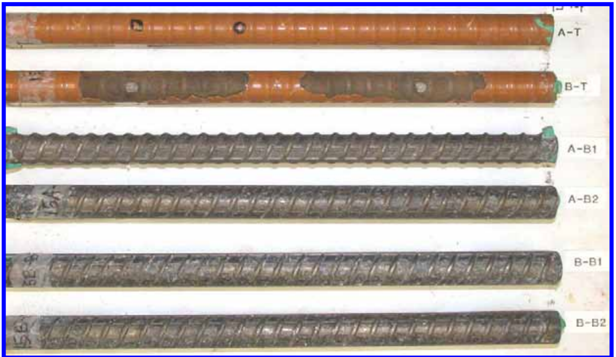
Figure 89. Slab #15 after autopsy
