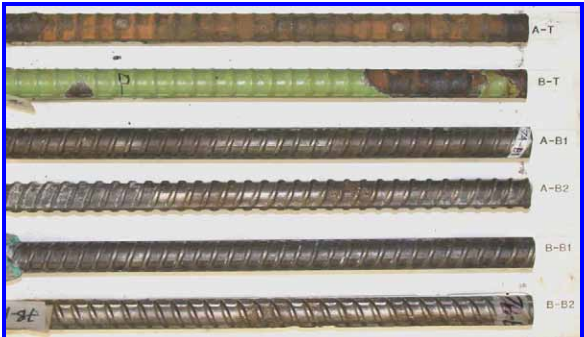
Figure 65. Slab #7 after autopsy
