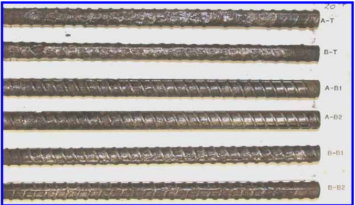
Figure 104. Slab #20 after autopsy
