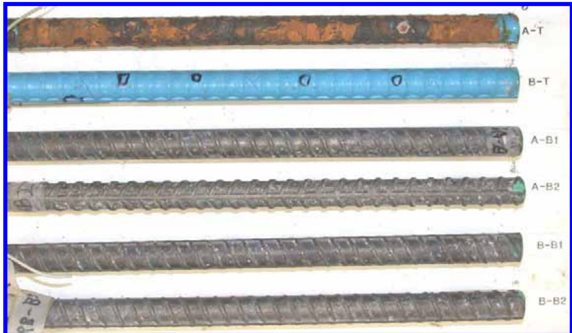
Figure 62. Slab #6 after autopsy
