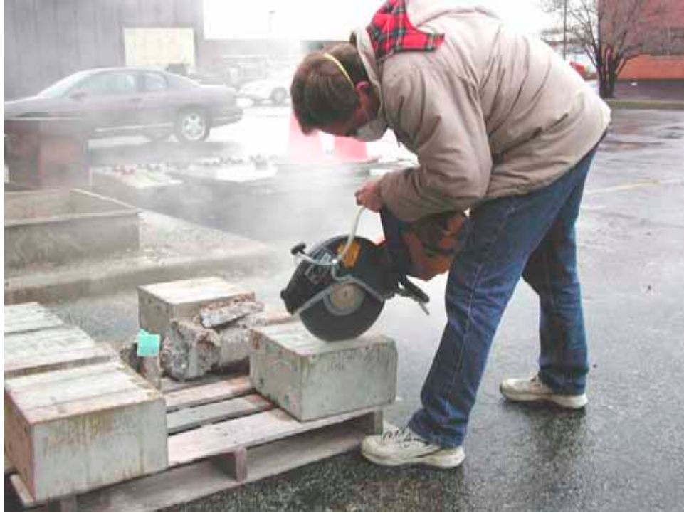
Figure 27. Cutting a test slab with a gas-powered saw
