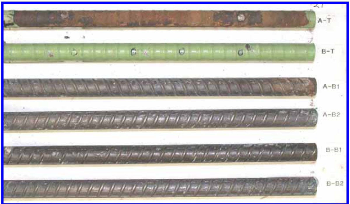
Figure 116. Slab #24 after autopsy
