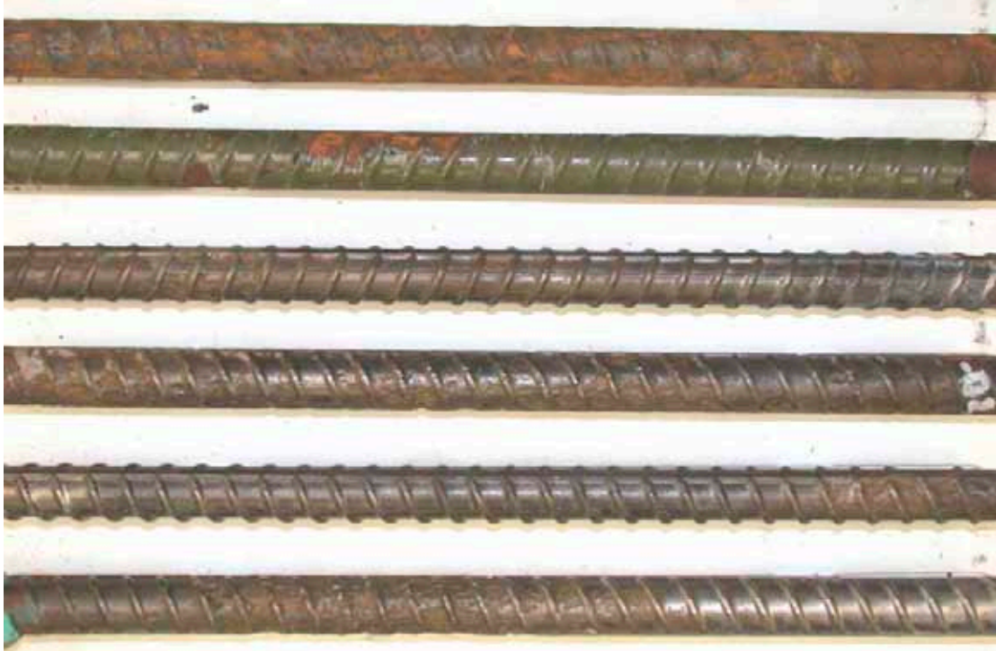
Figure 37. Photograph of autopsied bars extracted from slab #18 (ECR top-black bar bottom)
