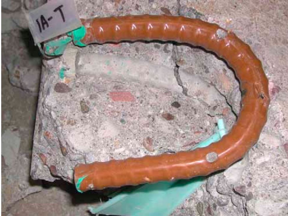
Figure 31. Typical condition of a bent ECR with good performance (slab #1—top left bar)
