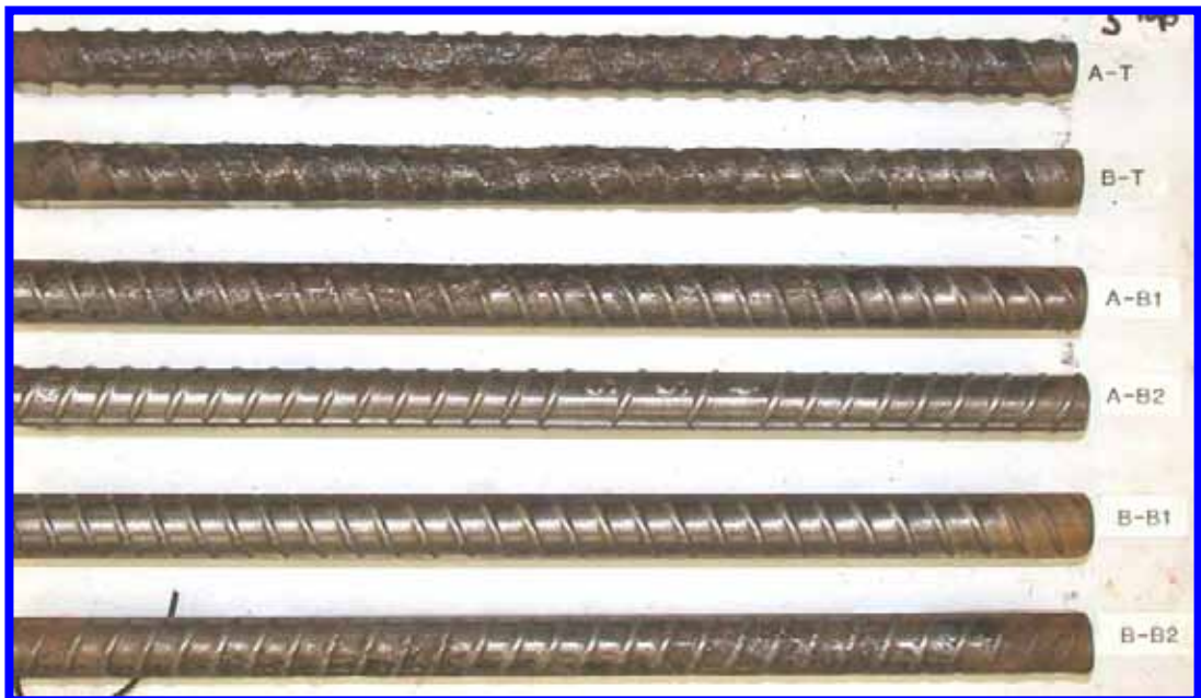
Figure 59. Slab #5 after autopsy
