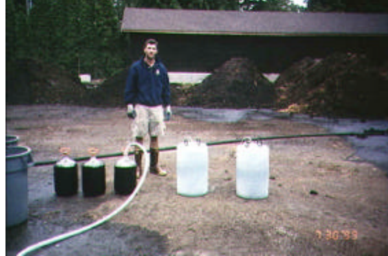
Pasteurization Containers Filled w/Runoff
