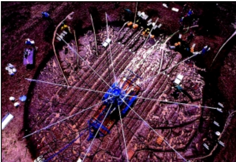
A rainfall simulator can provide quick runoff data at a lower cost than collecting natural storm events. However, if a very intense storm event is simulated after tillage the results can be misleading. This rainfall simulator and test plot at Cottonwood, South Dakota, enabled technicians to measure water runoff rates and collect soil samples in a WEPP cropland field study.
