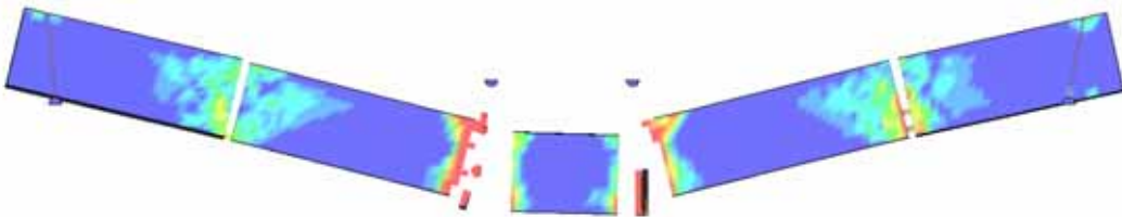
Figure 171. Plain concrete damage fringe t = 30 msec (user Windows).
