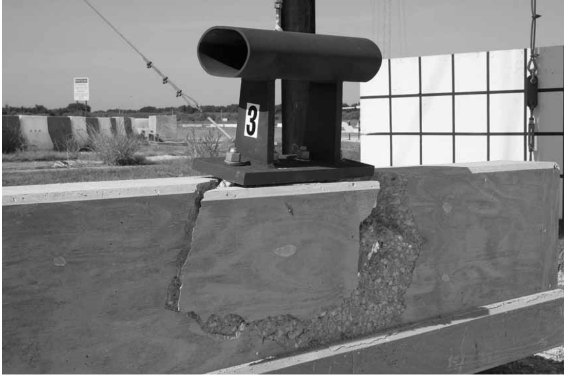
Figure 87. Parapet damage after test P3.
