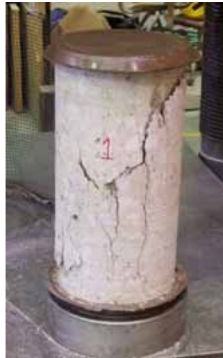
Figure 14. Concrete cylinder tested as part of the bogie vehicle impact test series.
