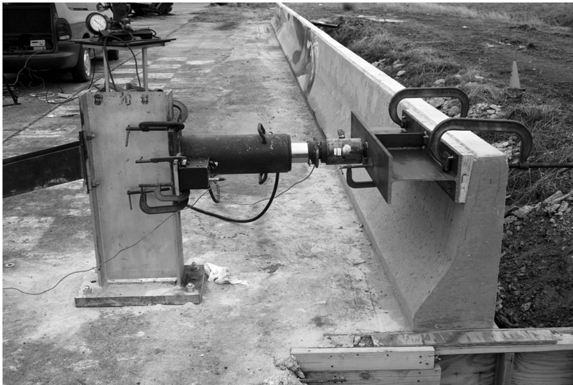
Figure 132. Test setup for static load tests on safety-shaped barriers.
