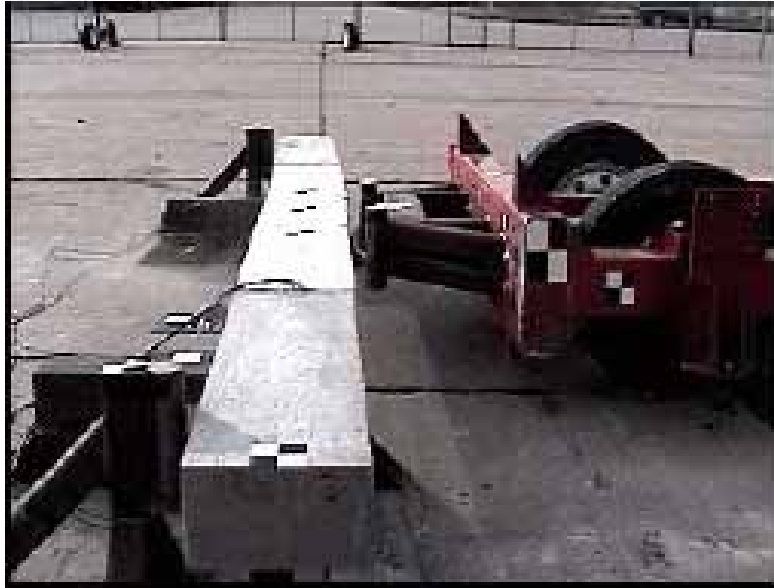
Figure 77. The beam rebounds when impacted at 8.6 km/h (5.3 mi/h), pushing the bogie vehicle backward.
