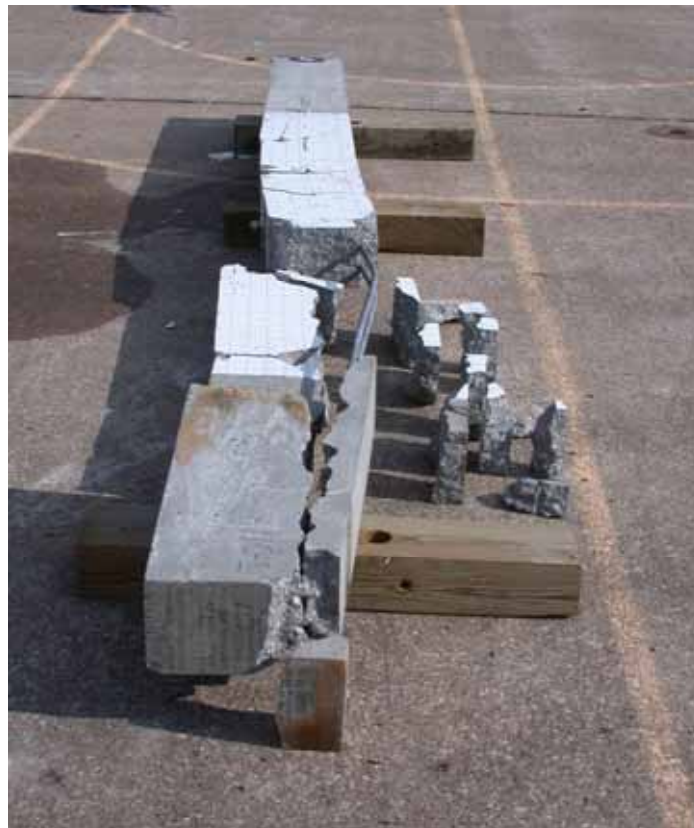
Figure 72. Damage dominates one side of the beam impacted at 15.9 km/h (9.9 mi/h).
