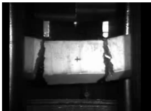
Figure 50. Six of the eight plain concrete specimens initially failed with two major cracks in the impact regime.
