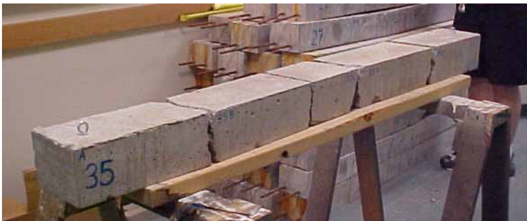
Figure 53. Four of the eight plain concrete specimens ultimately break into five pieces.
