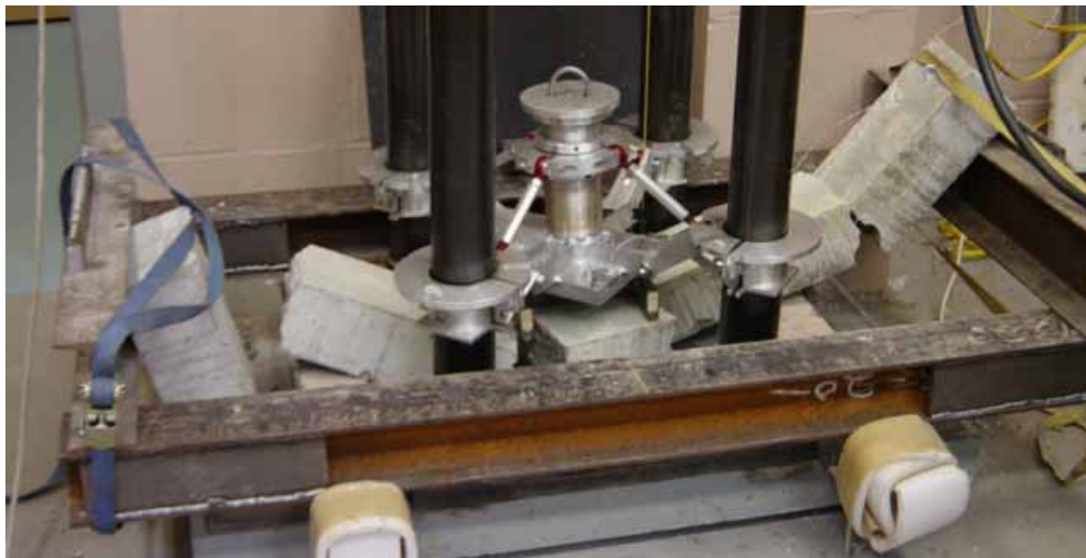
Figure 52. All plain concrete specimens impact the bottom of the test fixture.
