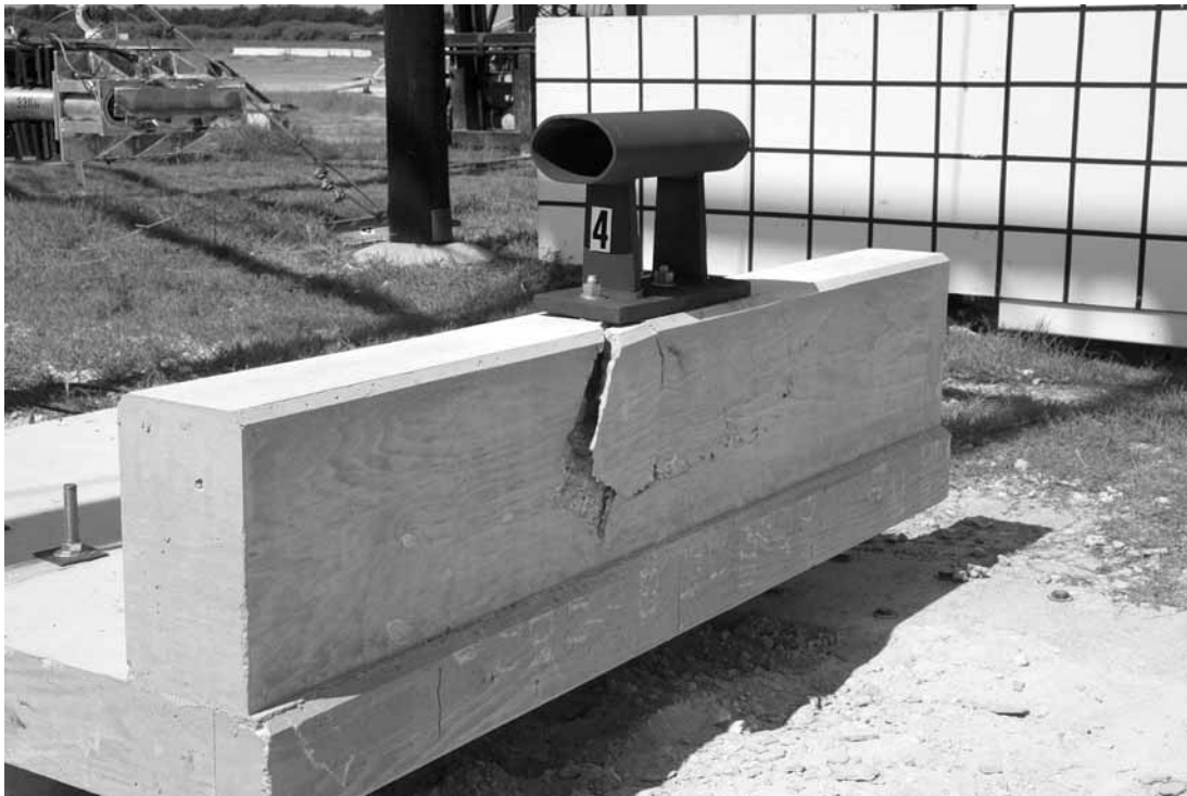
Figure 88. Parapet damage after test P4.
