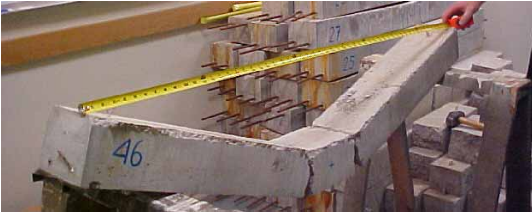
Figure 63. The damage mode measured for half of the under-reinforced beam specimens is two major cracks beneath the impactor points, without rebar breakage.
