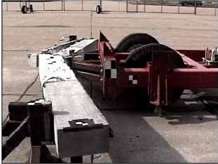
Figure 71. The beam tested at an impact velocity of 15.9 km/h (9.9 mi/h) exhibits inclined shear cracks, localized crushing, and bond failure.
