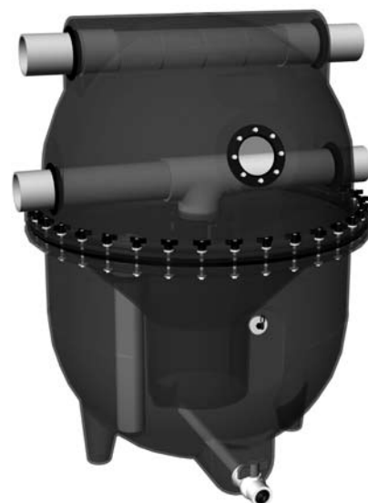
PolyGeyser “Pneumatically Washed” Drop Bead Filter, Model DF-15. This filter contains 6 ft 3 of Enhanced Nitrification (EN) Bead Media and is designed to provide complete biofiltration and clarification for systems being fed up to 9 lbs of 35% protein feed per day.
