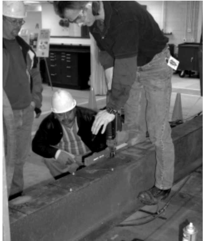
A lab technician drives PAFs into a steel beam at THFRC's Structures Lab.
