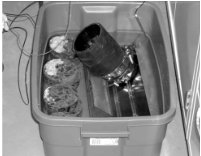
The rapid migration test, pictured here, is a new method for predicting chloride ion penetration in bridges and pavements.
