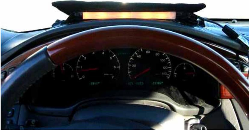
Figure 3. Photo. Light source used to control driver light adaptation level.
