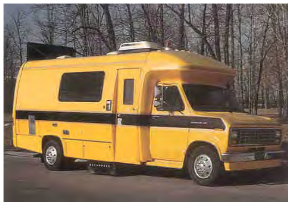
Figure 2. K.J. Law Engineers DNC 690 profiler with a motor home body.
