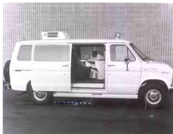
Figure 3. K.J. Law Engineers DNC 690 profiler housed in a van.
