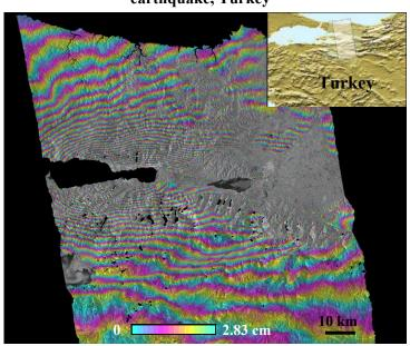
InSAR refines our understanding of the earthquake cycle through mm-level interseismic and coseismic vector deformation maps along faults and plate boundaries.
