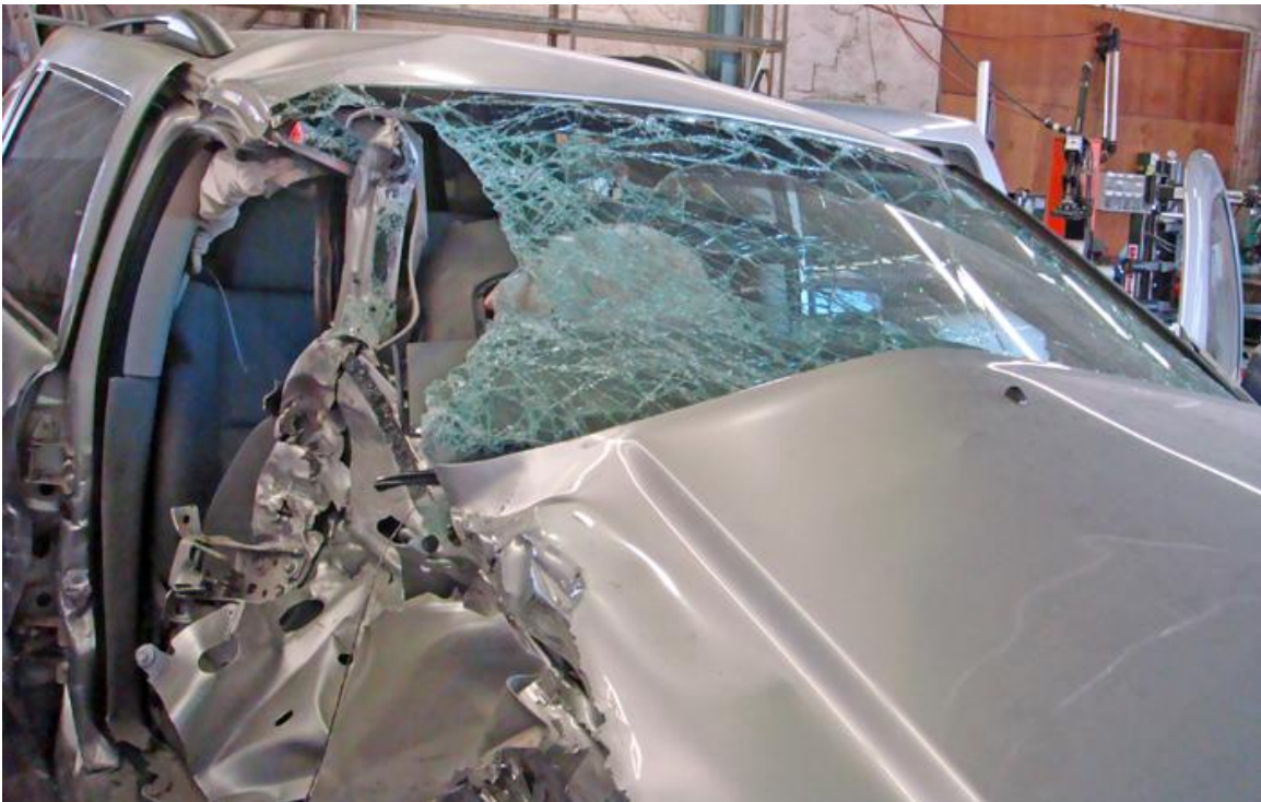
Photo shows the crash energy impact location.
