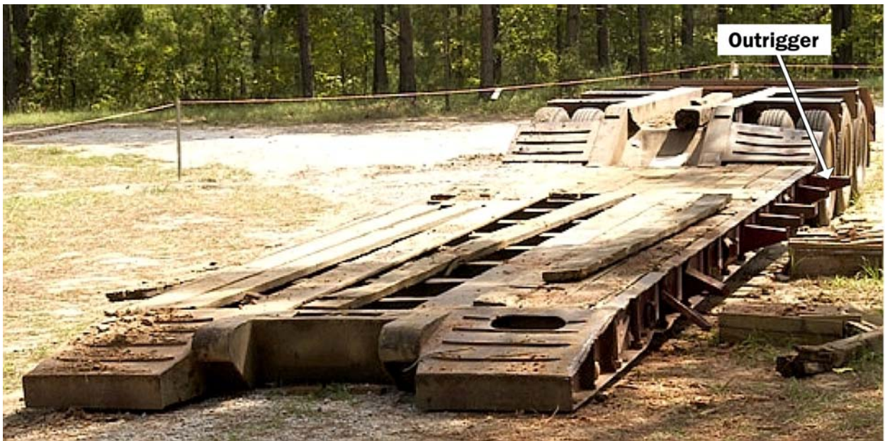
Figure 2-2. Lowboy after removing excavator
