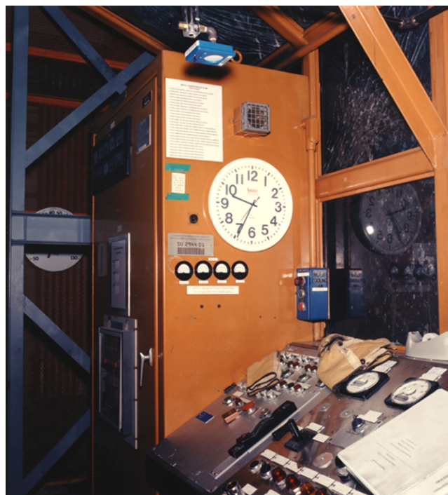
Exhibit #4. Skull Caster Furnace Control Panel Showing Clock Stopped as a Result of the Accident
