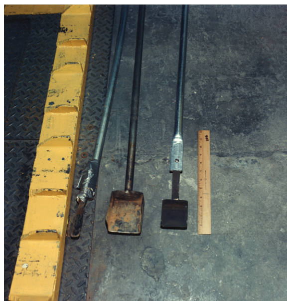
Exhibit #3. Metal Tools Used To Probe and Break Up the NaK Spill
