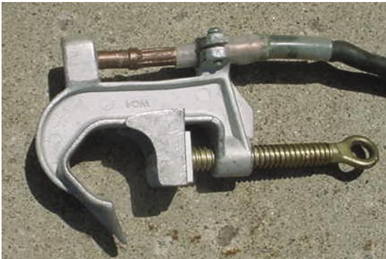
Figure 2: This clamp (bus type) was connected to the conductor (“hot end”).
