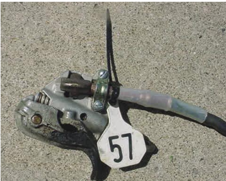
Figure 3: This clamp (duckbill type) was connected to the steel (“cold end”).
