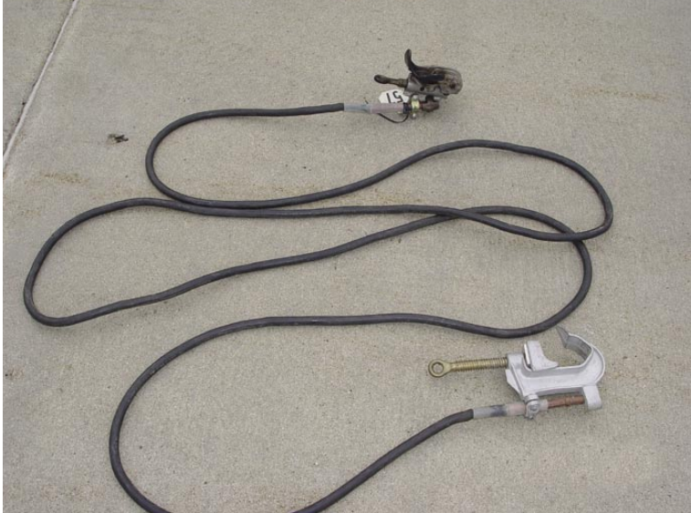
Figure 1: Ground lead (2/0 cable, 20 feet, 6 ½ inches long) that was connected between the A phase of the Watertown-Granite Falls 230-kV transmission line and the steel at Structure 38/1. At the time of the accident, the victim disconnected the “cold end” while the “hot end” was still connected to the A phase conductor. This type of grounding assembly is designed for bus-bar or phase-to-phase grounding applications.
