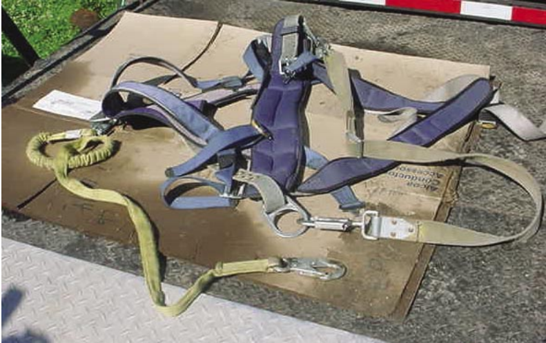
Figure 4: Harness, body belt and lanyard worn by victim at the time of accident.
