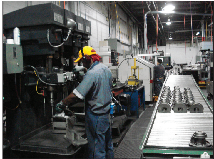
Monitoring a worker's exposure to airborne metals during a high-speed drilling operation
