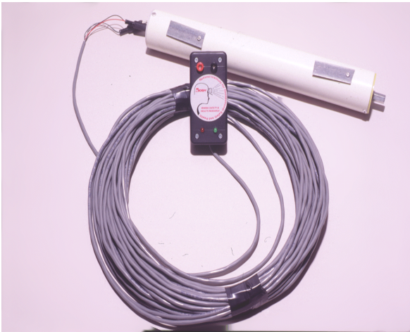
Figure 2. RMSS, cable and read-out box.
