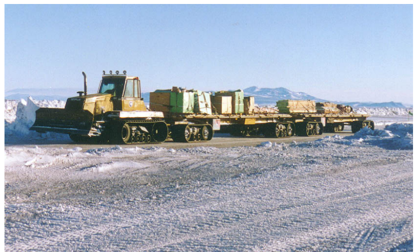
Figure 4. Tandem tracked trailers on traverse from Marble Point to McMurdo.
