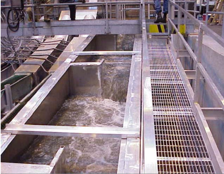
Figure 3. Picture of experimental fishway operating with overflow/orifice weirs in place.
