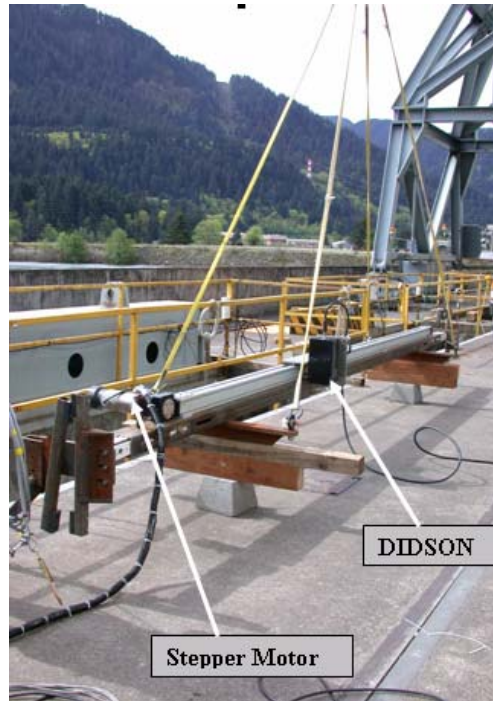
Figure 2.12. Traversing Beam and DIDSON Assembly Deployed in the Gatewell Slots of Intakes at Units 13 and 17. The stepper motor that moved the DIDSON along the beam is on the left end of the beam and the moving plate with the DIDSON attached is in the middle of the beam. The beam was deployed by riggers using the TIE crane.
