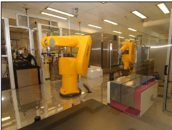
Housed at the NIH Chemical Genomics Center, these Kalypsys robots perform precision plate handling for high throughput screening. (Photo courtesy of NHGRI)
